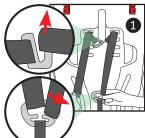
7. Pull the up-front harness adjustment strap as far as it will go. This will lock the splitter plate into the base of the seat 4.
